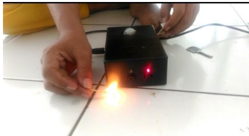
Figure 4. LM35 temperature sensor testing
