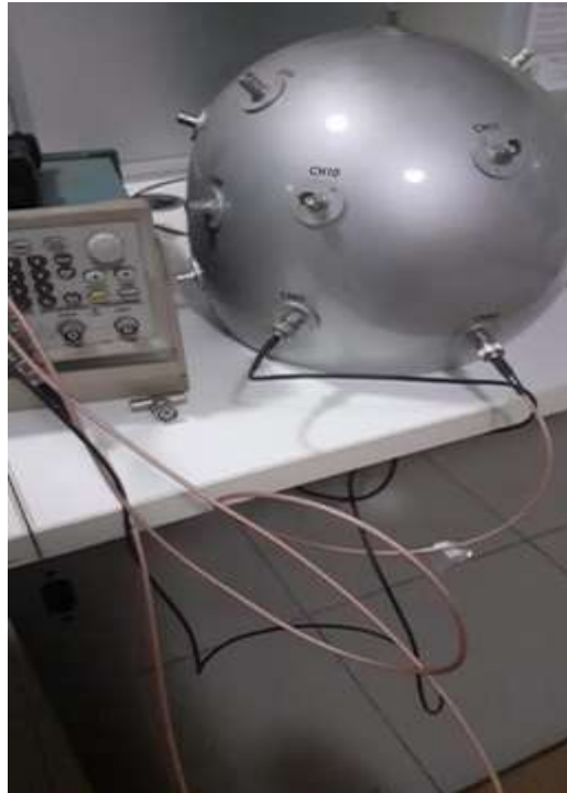
Figure 3. Brain Scanning System Based on 16-Electrode ECVT
