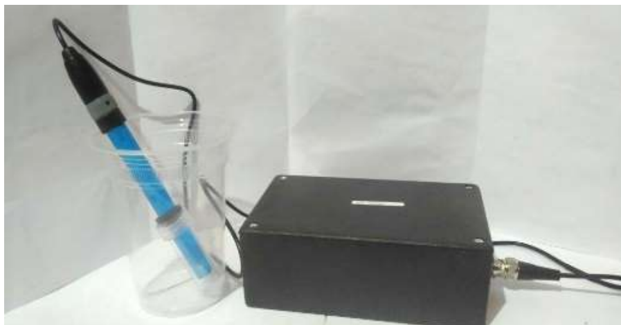
Figure 2. pH Meter - showing the assembled device with probe and Arduino unit
