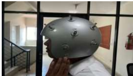
Figure 1. 16-Electrode ECVT Brain Scanning System
