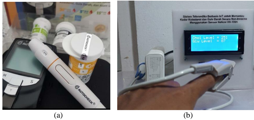
Figure 1. Blood sugar level measurement tools: (a) Invasive method and (b) Non-invasive method
